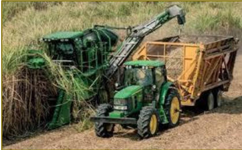
*Mechanized Harvester feeding cane into 10+ MT trailer/tender*
